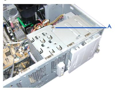
Figure 4 - 18: HDD Bracket Screw
